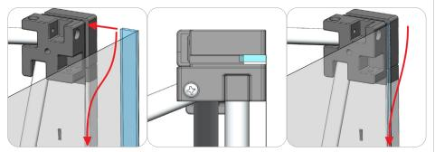
As an optional feature, the front printed graphic may have end cap graphics with silicone edge. Pull the end cap silicone edge to the top of the back corner hub. Start to press in the SEG into the hub and work your way down the side channel. Do the same for the opposite end cap.
